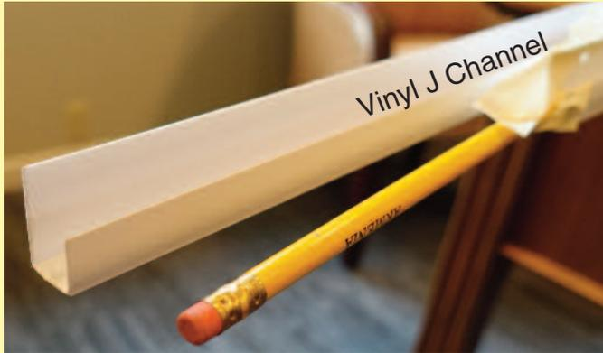
*Any other material could also be used for the top horizontal support; such as wood moulding, aluminum extrusion, small diameter PVC pipe, or anything else.*
